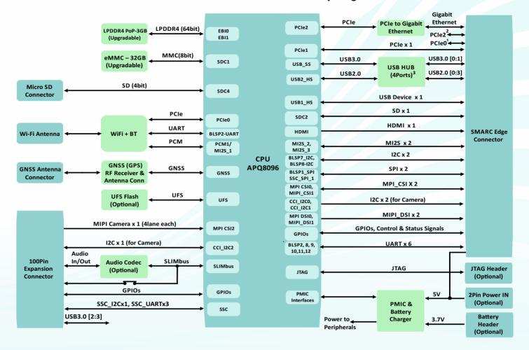
Note1: If On-SOM WIFI+BT is used, PCle0 cannot be used on SMARC Edge Note2: If On-SOM Ethernet PHY is used, PCle2 cannot be used on SMARC Edge
